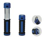
30+1WLED Rechargeable Working Light 30PCS SMD 3528 bright LED light.,1WLED on the top as spotlight., LED chargingi indicator.,using 3.7V 1200mA lithium battery., Magnet and hook in the bottom., AC-DC adapter and DC12V cigarette plug charger,
